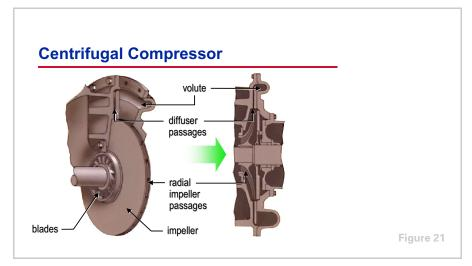
The center, or eye, of the impeller is fitted with blades that draw refrigerant vapor into **radial passages** that are internal to the impeller body. The rotation of the impeller causes the refrigerant vapor to accelerate within these passages, increasing its velocity and kinetic energy.
